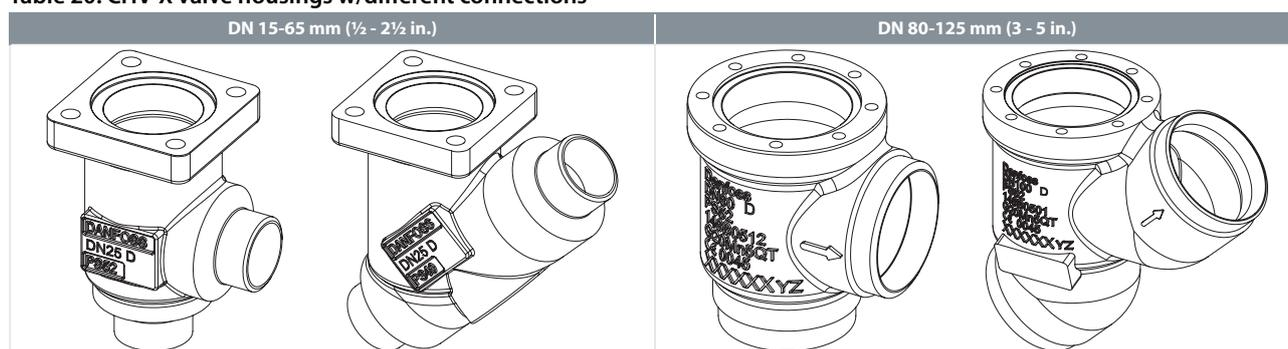
**Table 21: CHV-X valve housings w/different connections**
