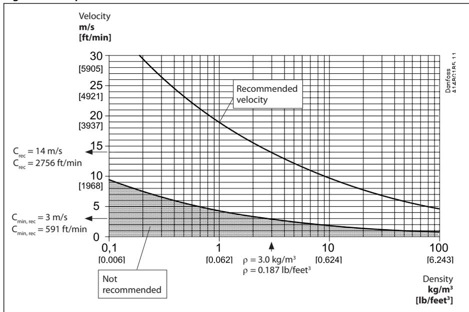
Knowing that  $V = 1000 \text{ m}^3/\text{h}$  (1160 gpm) fig. 2 gives the following choices:
