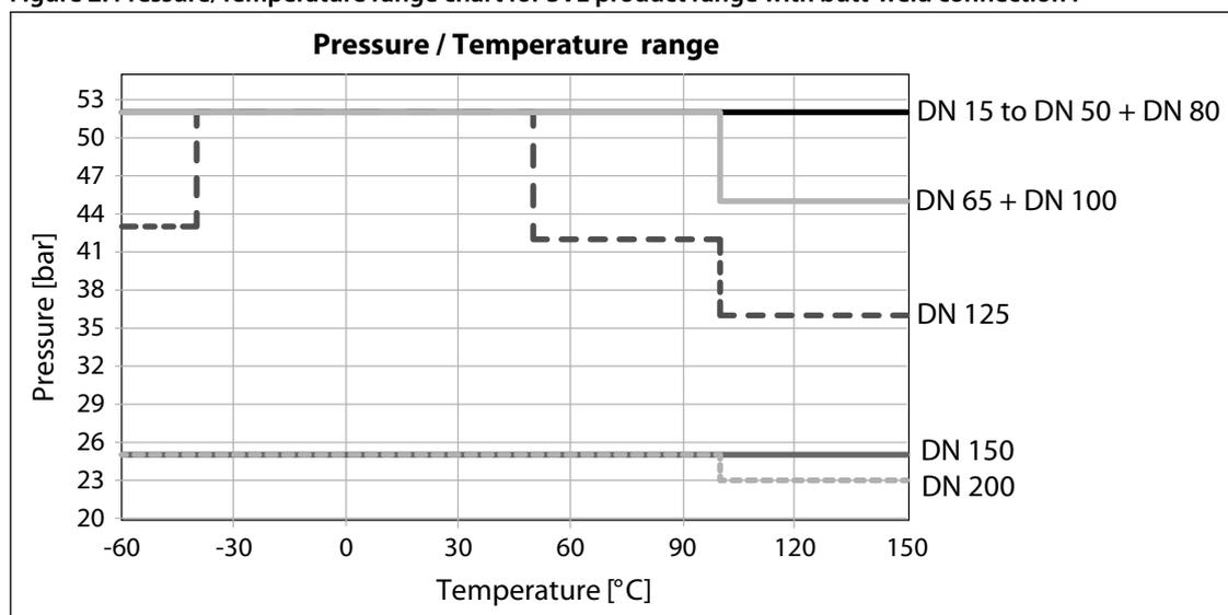
**For valve sizes DN 15 to DN 50 and DN 80:**
