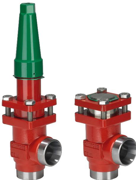
SCA-X are check valves with a built-in stop valve function. CHV-X are check valves only. SCA-X/ CHV-X are available in angleway versions. The valves are designed to open at very low differential pressures, allow favourable flow conditions and are easy to disassemble for inspection and service.
