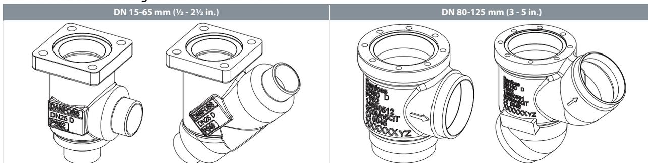
Table 17: SVL valve housings w/different connections
