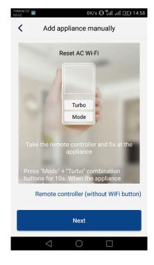
5. Select WiFi hotspot of the AC unit. Its name should correspond to the MAC address of Wi-Fi module (you can find this information on the cover of Wi-Fi module in the unit, it is combination of letters and numbers), the password is "12345678". After filling in all required information, press "Next".
